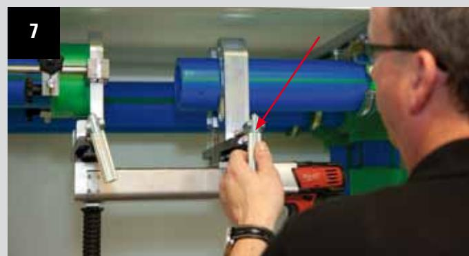
Never clamp so tight that deformations appear. Additionally, with the fitting support, all fittings are supported. The support is mounted on the clamping jaw for fittings. (Fig.8)
