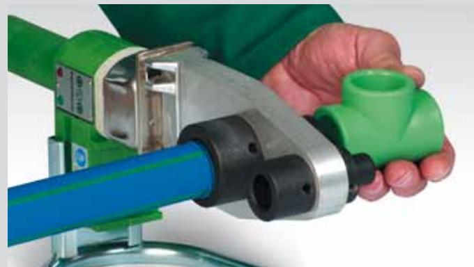
Heating-up of pipe and fitting
