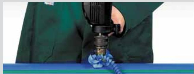
Drilling through the pipe wall
