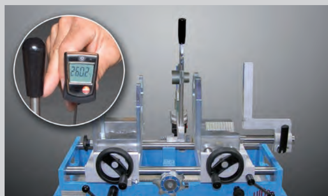
Temperature control - aquatherm welding machine
