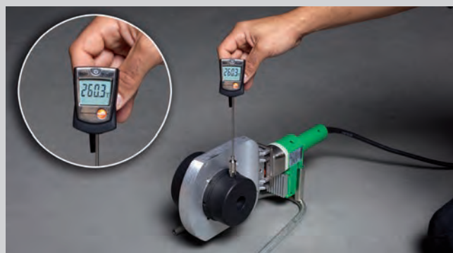
Temperature control - aquatherm welding device (1400 W)
