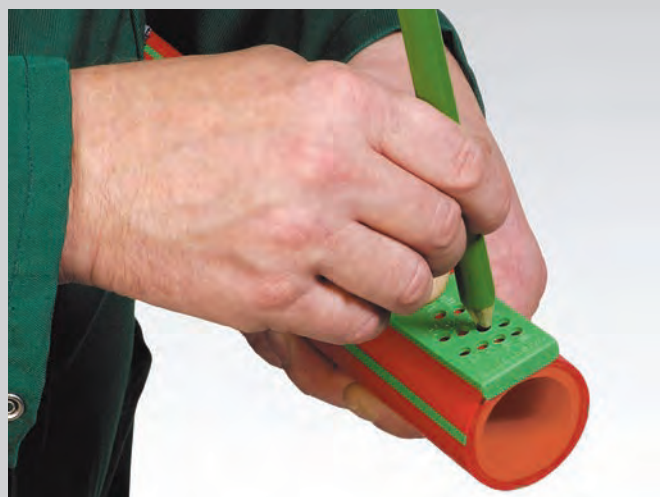
Marking of the welding depth
