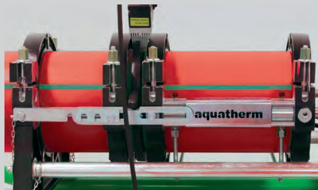
Positioning of heating element
