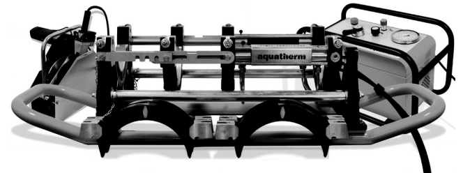
Check performance of the welding machine and heat it up.
