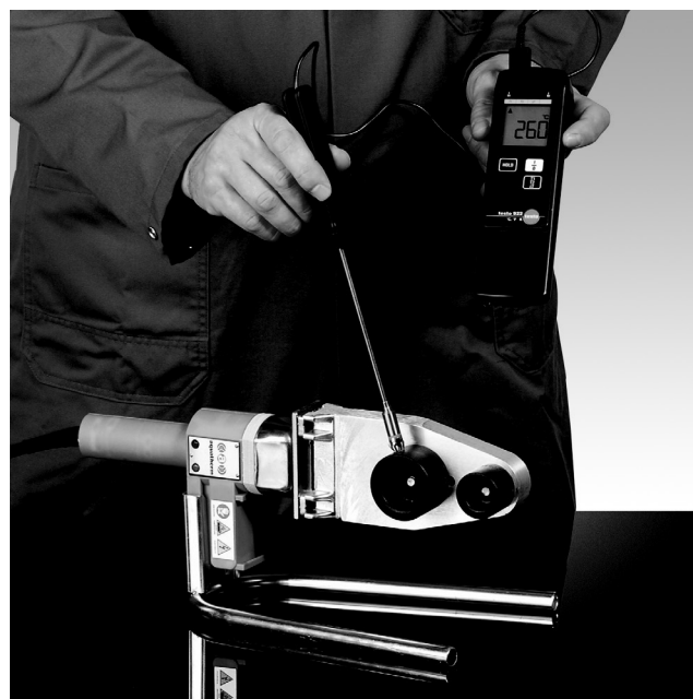
Temperature control with a thermometer.
