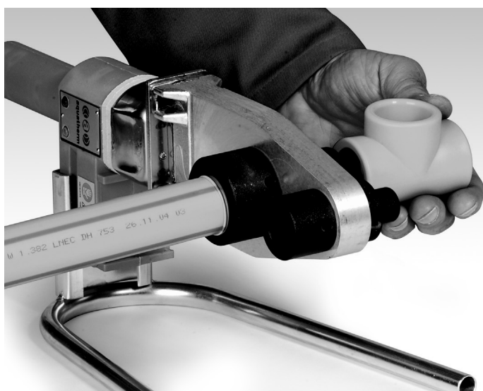
Heating up of pipe and fitting
