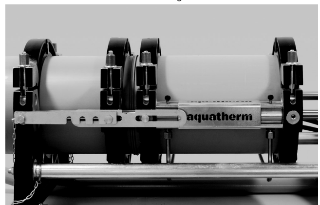
Join the pipes, cool down under pressure
