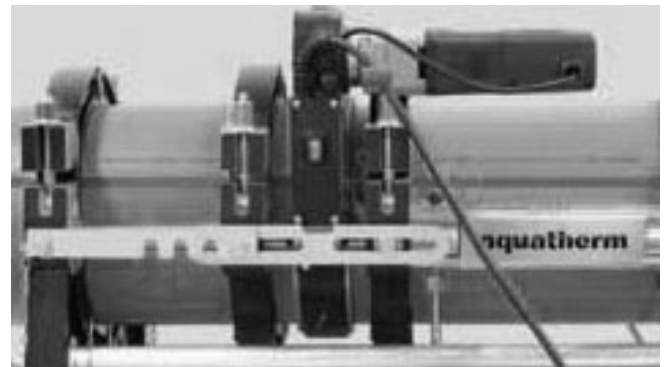
The part to be welded are fixed and aligned respectively, the milling machine is used
