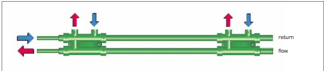
The flow and return connections of heating pipes to the aquatherm-distribution block are with aquatherm PP-R pipes of an external diameter of 20 mm. Used in conjunction with the aquatherm orange system-connecting bend (Art.-No. 85120) and the aquatherm orange system-radiator valves (Art.-No. 85102 or 85106), the outgoing 16 mm pipe connections are ideal for radiator connections.
