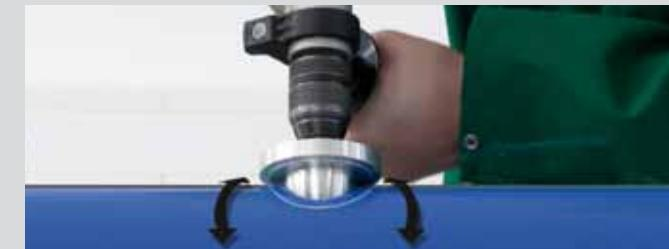
Removal of the oxygen barrier layer from the aquatherm blue OT-pipe
