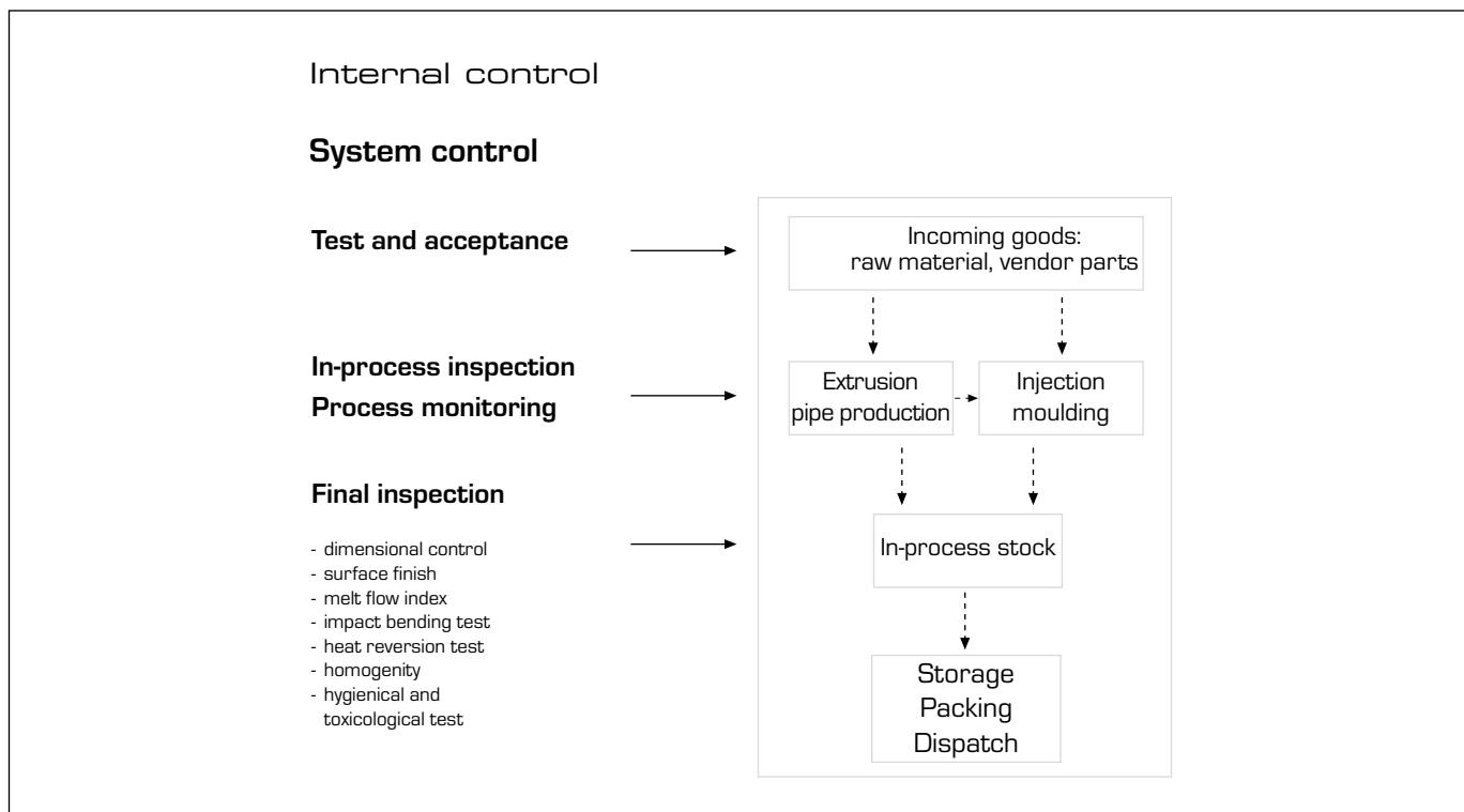
In addition to the permanent internal quality control, an external control is made by i.e. SKZ, SAI, TGM, Hygieneinstitut.
