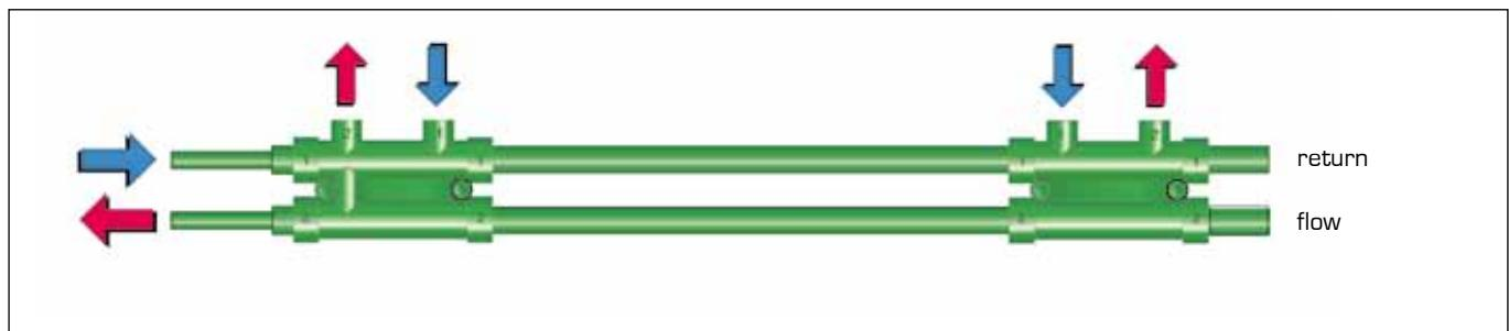
It is of no importance, where the heating flow or return is connected to the aquatherm orange system-distribution block. A simply turning of the distribution block adapts it to the appropriate specification.
