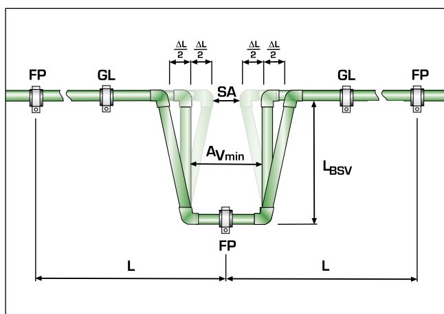
All bellow expansion joints for corrugated pipes designed for metal materials are unsuitable for aquatherm PP-R pipes.
