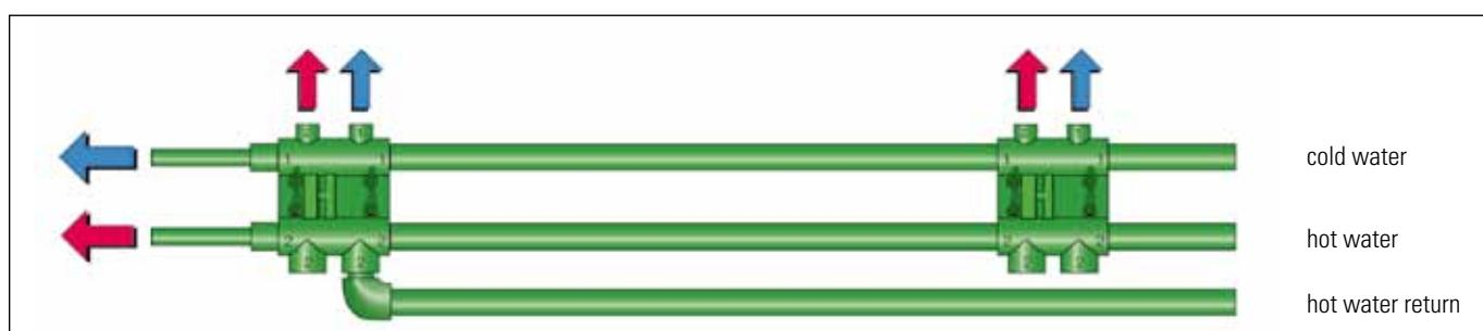
Reducers for further pipe systems can be welded directly onto the distribution block.
