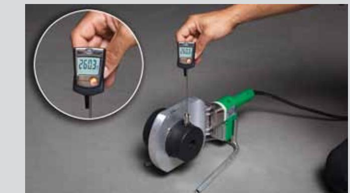
Measurement of temperature at the aquatherm manual welding device (1400W)
