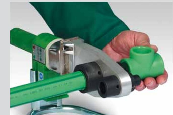
Heating-up of pipe and fitting
