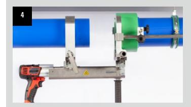
The two arrows of the jaws and the machine must be flush with each other. The jaws are to be fixed with the help of the clamping device (Fig. 5).
