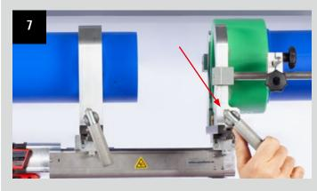
Never clamp so tight that deformations appear. Additionally, with the fitting support, all fittings are supported. The support is mounted on the clamping jaw for fittings. (Fig. 8)
