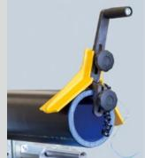
Chamfering of the front side in case of the OT and UV pipe
