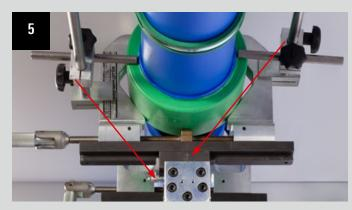
Align the pipe so that the rear marking is flush with the inner edge of the clamping jaw. The front marking identifies the welding depth (Fig. 6).
