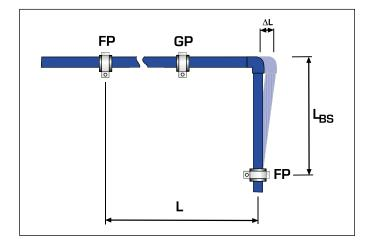
Calculational determination of the bending side length
