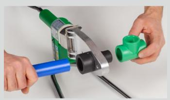
Heating-up of pipe and fitting
