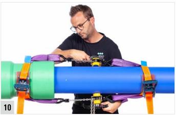
Pull the push-fit fitting onto the pipe end up to the marked insertion denth
