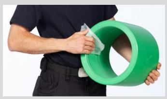
lean the electrofusion socket's inner surface with a lint-free cloth or paper. Remove moisture that may occur **immediately before the welding process** again.
