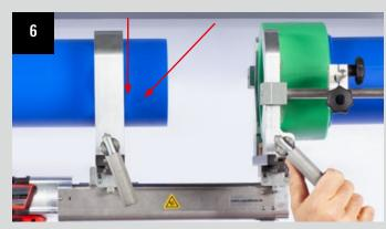
Lock pipe and fitting by using the front adjusting screws. (Fig. 7)
