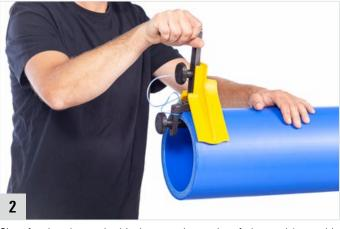
Chamfer the pipe end with the aquatherm chamfering tool (see table minimum chamfer length).
