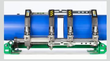
Divide the machine slide, remove heating element
