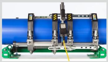
Positioning of heating element
