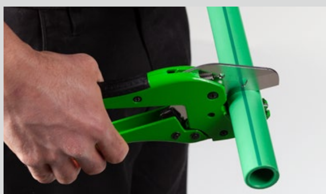
Cutting of the pipe
