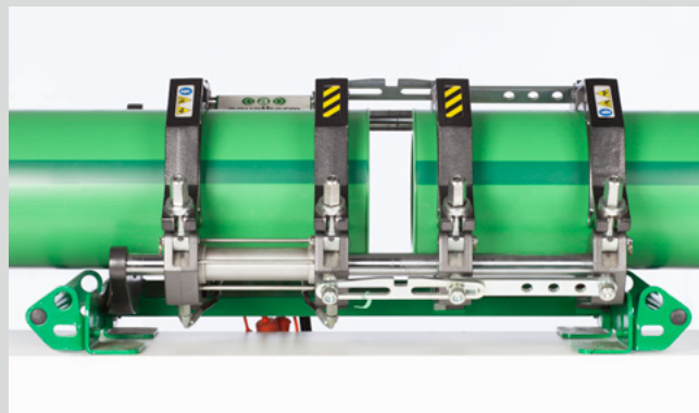
Divide the machine slide, remove heating element
